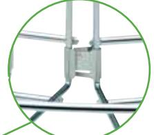
Very easy to make angles on site. Just cut and bend the mesh tray to the desired angle and use the fast-fix locking-clips to fix and secure the wires
